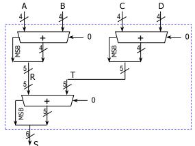
• The figure below depicts the internal architecture of the 4-bit adder and the 5-bit adder. The full adder circuit is also shown.
